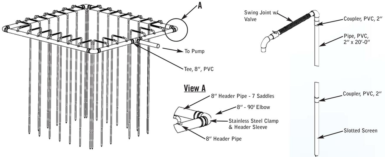
The wellpoint system is used to lower the water table to allow construction of buildings and civil works. All pipes shown bring water from the ground to the suction port in the pump. Discharge from the pump is then either directed to a canal or catch basin depending on site conditions.
