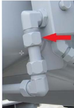
2. Remove 90° elbow from lube assembly manifold and clean threads on the manifold. Inspect the threads after cleaning and ensure there is no damage.
